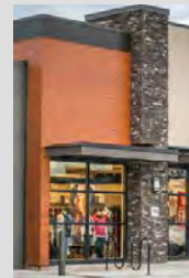
Desired design for a retail building. The color palette includes natural and earth tones. Building uses brick (primary) and EIFS (secondary), and architectural details that breakdown the facade to human scale. There are varying building planes and heights.
