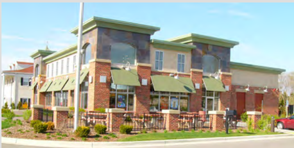
Desired design for a retail building. The color palette includes natural and earth tones. Building uses brick (primary) and EIFS (secondary), and architectural details that breakdown the facade to human scale. There are varying building planes and heights.
